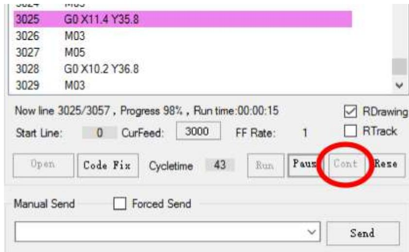
To stop the process click the Reset. This button has two important features: 1) When creating the code even when you stop it you cannot move the laser without clicking the Reset. 2) You cannot load another G-code without clicking the Reset.
